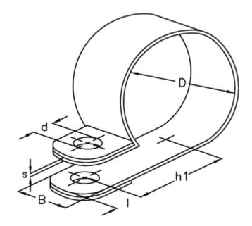
$\begin{array}{ll} d & = 5.3 \\ \text{Diameter D} = 51 \\ \text{h1} & = 32.3 \\ \text{I} & = 5.0 \\ \text{s} & = 0.5 \\ \text{Width B} & = 12 \\ \end{array}$
